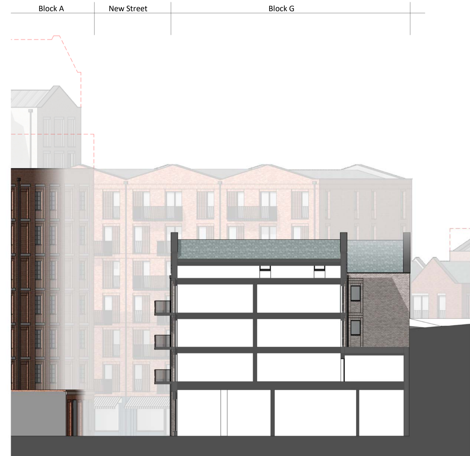
4 Block G - East Elevation (inner)
